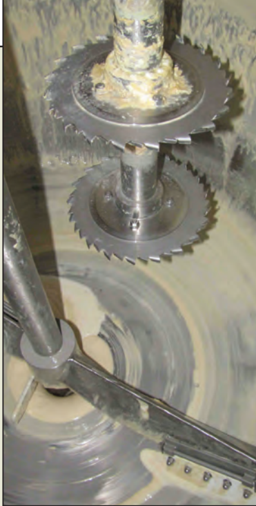
FIGURE 2. In production, dual disperser blades apply high shear, while a two-wing anchor scrapes the vessel's sidewall and bottom, promoting flow, then complete discharge
