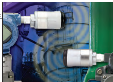
FIGURE 3. Emerson's Smart Wireless THUM Adapter can retrofit an existing two- or four-wire HART device. It enables wireless transmission of measurement and diagnostic information that was previously unavailable
