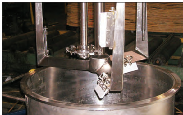
FIGURE 3. In-plant tests were conducted with a mixer equipped with a high speed disperser and an anchor designed to generate axial and lateral flow
